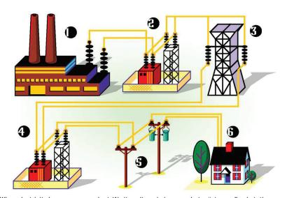
When electricity leaves a power plant (1), its voltage is increased at a "step-up" substation (2). Next, the energy travels along a transmission line to the area where the power is needed (3). Once there, the voltage is decreased or "stepped-down," at another substation (4), and a distribution power line (5) carries the electricity until it reaches a home or business (6).
